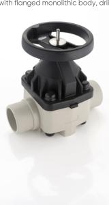
Diaphragm valve with flanged monolithic body, drilled ANSI B16.5 cl.150 #FF
